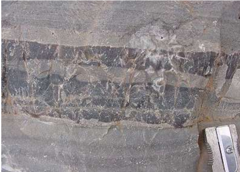
Black chert bands formed of silica from marine sponges, in the Westleigh Limestone and used in buildings. © SJ Parkhouse
